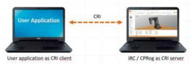
For the development of applications, the user application can interact with igus Robot Control / CPRog. The commands are then executed by the simulated robot arm.
