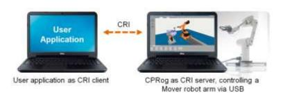
Robots without embedded control, e.g. the Mover robots, can also be commanded using the CRI interface. Simply connect to the PC software like in the simulation case.
